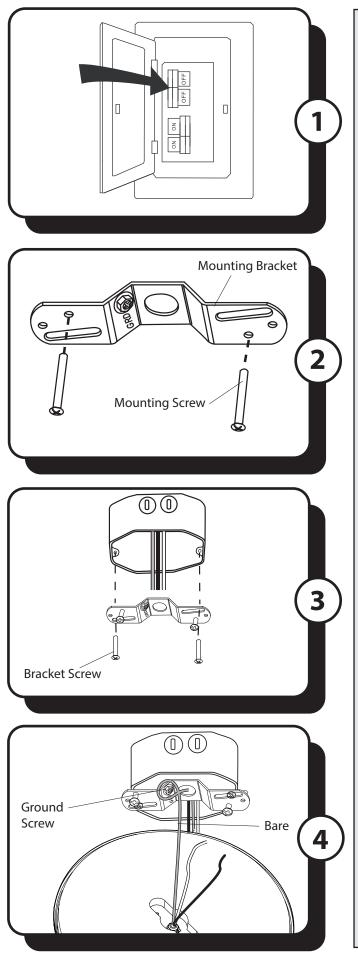
1.Turn OFF the electrical power at the main fuse or circuit breaker.
