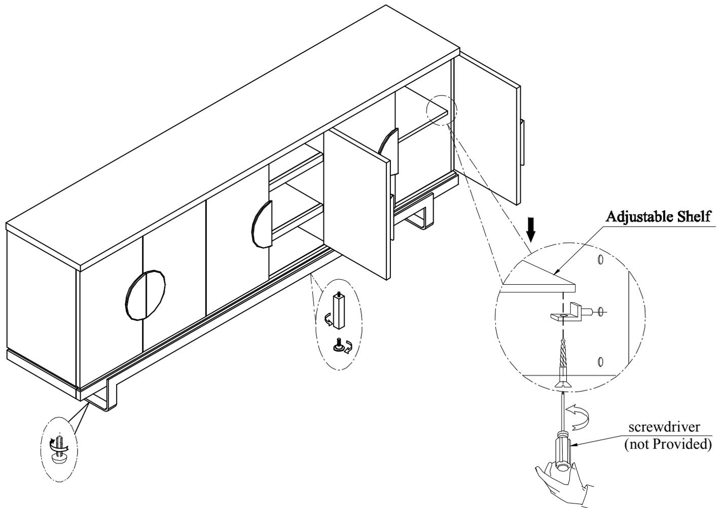
**Adjust levelers if needed, to level case on uneven floor**
