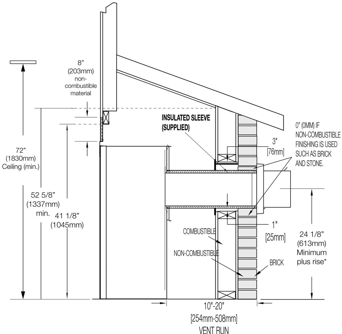
**Horizontal vent sections:** A minimum clearance of 3" (76mm) on the top outside of the enclosure and 1" (25mm) on the sides and bottom outside of the enclosure all around the vent pipe on all horizontal runs to combustibles is required. Horizontal vent sections within enclosures require a minimum clearance of 3" (76mm) at the top of the vent pipe.
