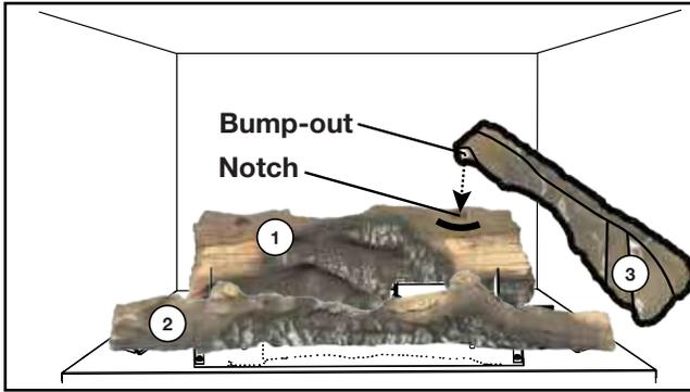
3. Place the bumpout on Log #3 (W135-0688) into the right notch of Log #1 resting the opposite end onto the lower portion of the media tray.
