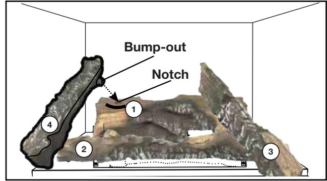
4. Place the bumpout on Log #4 (W135-0687) into the left notch of Log #1 resting the opposite end onto the lower portion of the media tray.
