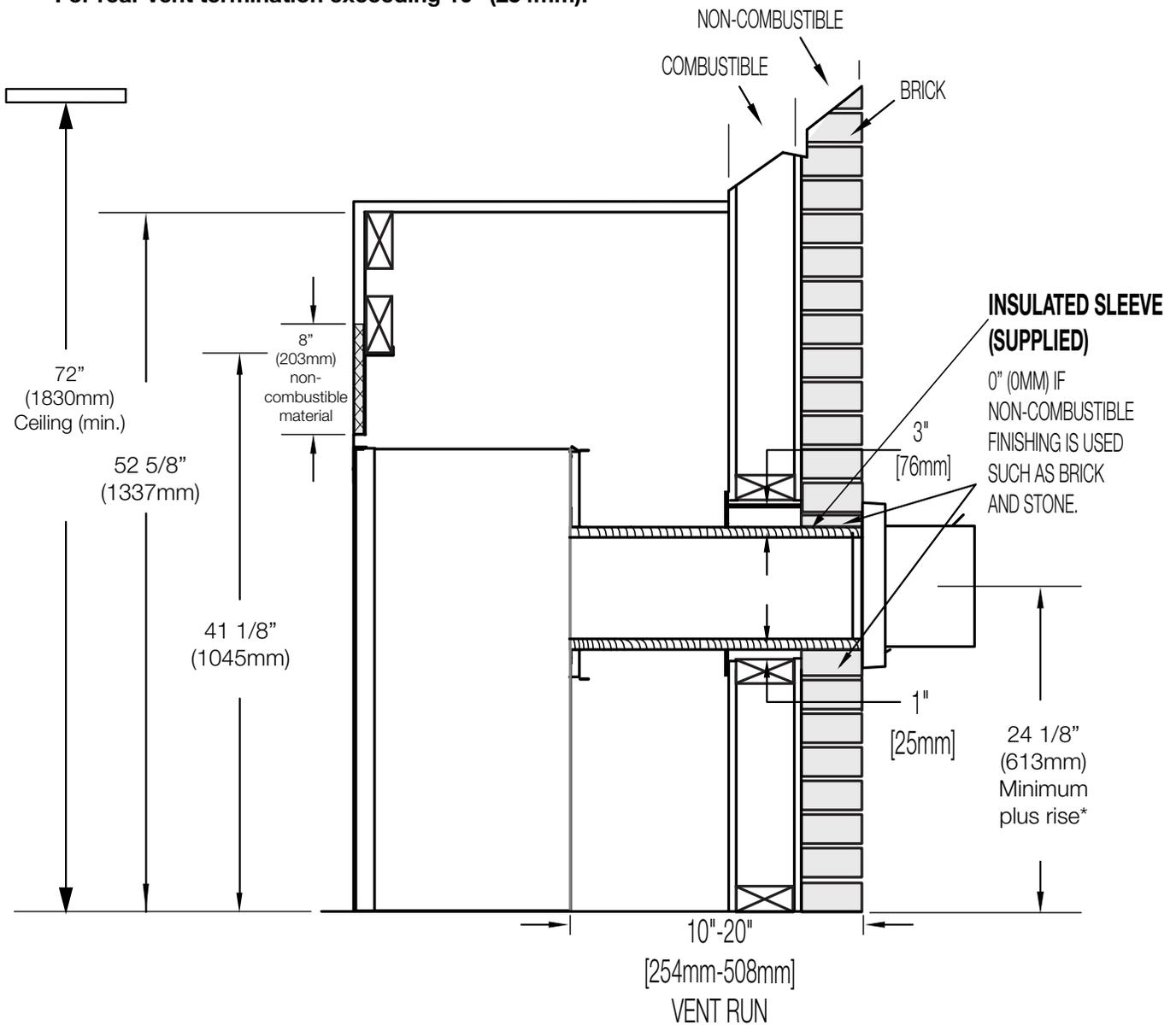
**Horizontal vent sections:** A minimum clearance of 3" (76mm) on the top outside of the enclosure and 1" (25mm) on the sides and bottom outside of the enclosure all around the vent pipe on all horizontal runs to combustibles is required. Horizontal vent sections within enclosures require a minimum clearance of 3" (76mm) at the top of the vent pipe.
