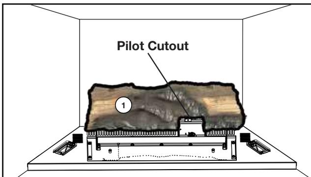
1. Place Log #1 (W135-0685) over the pilot and behind the airflow covers.
