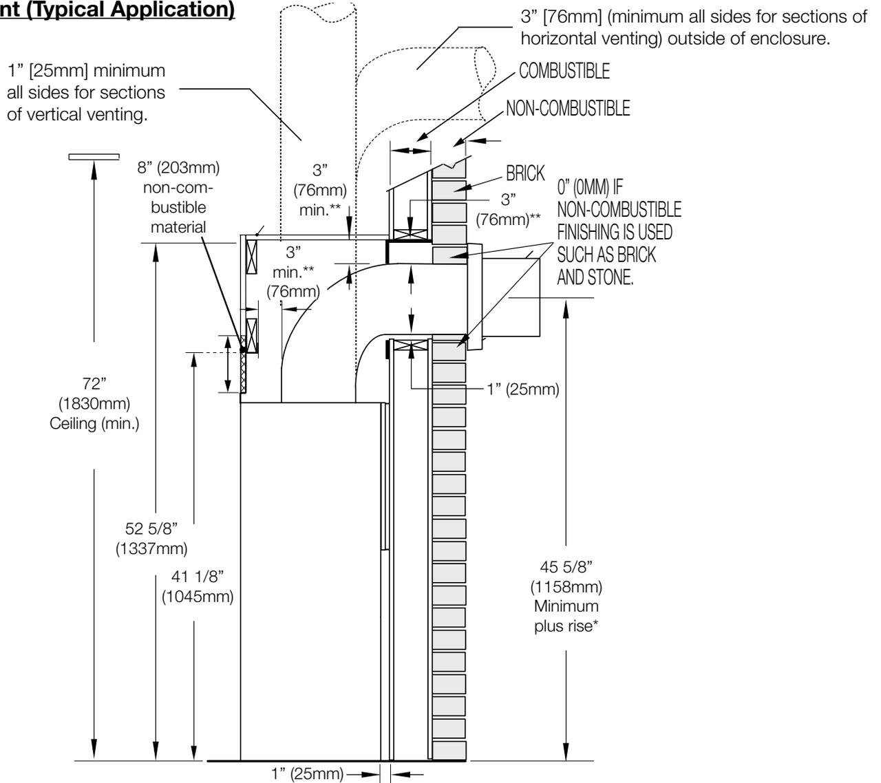
**Horizontal vent sections:** Outside of the enclosure, a minimum clearance to combustibles of 3" (76mm) on the top and 1" (25mm) on the sides is required all around the vent pipe on all horizontal runs. Inside the enclosure, horizontal vent sections require a minimum clearance of 3" (76mm) at the top of the vent pipe.
