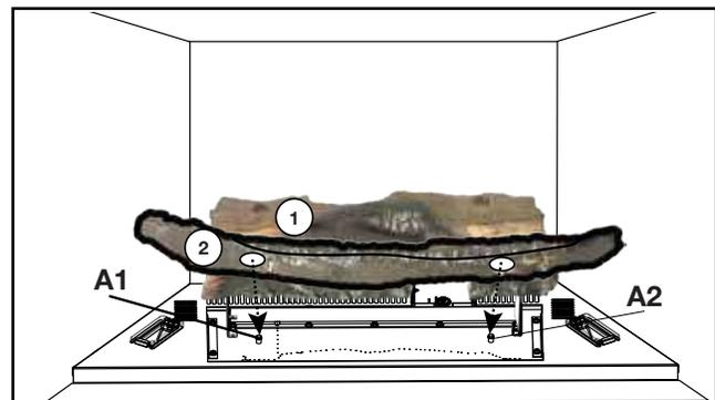
2. Place the locating holes of Log #2 (W135-0686) onto locating studs A1 and A2 (now is a good time to place the glowing embers).
