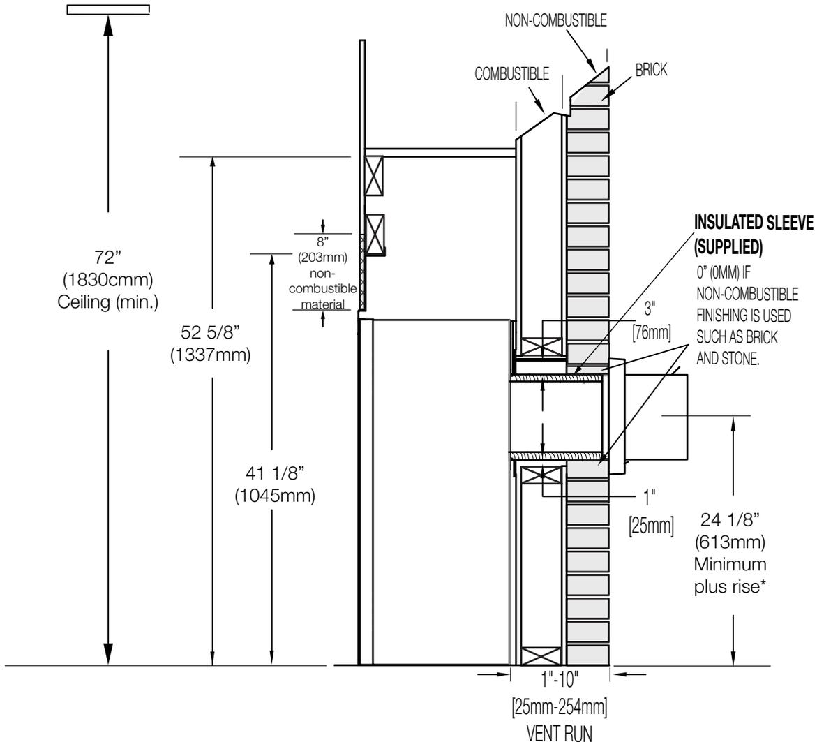
**Horizontal vent sections:** A minimum clearance of 3" (76mm) on the top outside of the enclosure and 1" (25mm) on the sides and bottom outside of the enclosure all around the vent pipe on all horizontal runs to combustibles is required. Horizontal vent sections within enclosures require a minimum clearance of 3" (76mm) at the top of the vent pipe.
