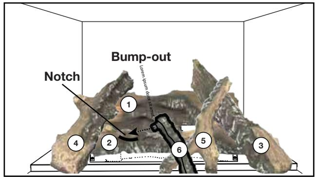
6. Place the bumpout of Log #6 (W135-0689) into the notch of Log #2 resting the opposite end onto the lower portion of the media tray.
