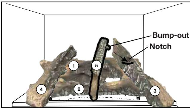
5. Place the bumpout on Log #5 (W135-0690) into the notch of Log #3 resting the "Y" onto the lower portion of the media tray.
