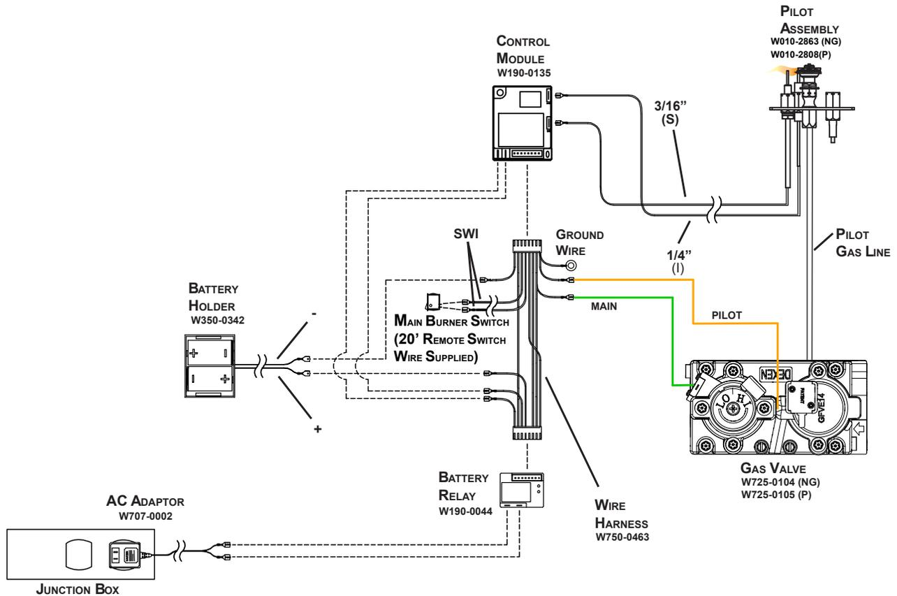
**NOTE: PLUG THE 3 VOLT AC ADAPTOR INTO THE APPLIANCE JUNCTION BOX TO SUPPLY POWER TO THE UNIT.**
