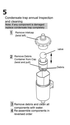
INSTALLATION INSTRUCTIONS Rolux® Vent System Condensate Trap Kit
