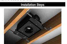
**Step 1.** Install Aculux new construction housing and gypsum board ceiling per the instruction sheet shipped with the recessed housing. Confirm the ceiling cutout dimensions are either 4-3/8" diameter for round apertures or 4-1/4" x 4-1/4" for square apertures. The aperture must be centered in this cutout to produce a uniform 1/8" gap between drywall and recessed housing.
