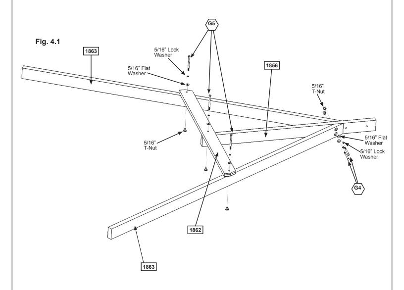
**B:** Attach (1862) SW Support to both (1863) SW Posts and (1856) SW Upright using 3 (G5) 5/16 x 4-1/2" Hex Bolts (with lock washer, flat washer and t-nut). (fig. 4.1)
