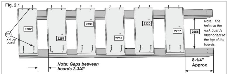
A: Lay 2 (2555) Rock Rails down, side by side with angled edges facing down. (fig. 2.1)
