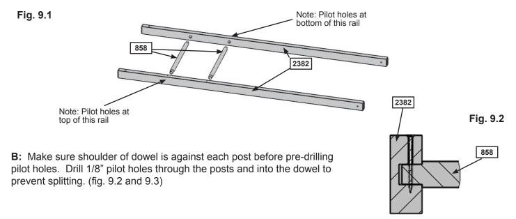
**C:** Attach (858) 1-1/8 x 18-5/8" Dowel to both posts with 2 (S2) #8 x 1-1/2" Wood Screws. Two screws are installed from top of the rails and the others from the bottom as shown in fig. 9.3.
