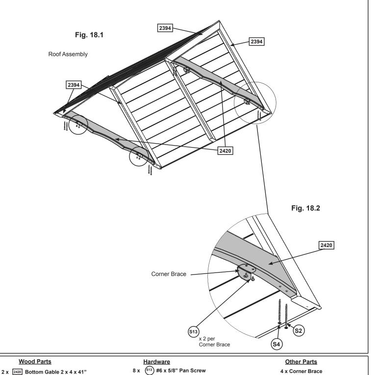
4 x (s4) #8 x 3" Wood Screw 4 x (s2) #8 x 1-1/2" Wood Screw
