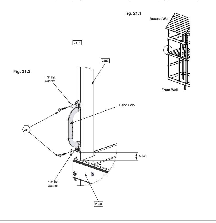
$\frac{\text{Hardware}}{2 \text{ x } \left\langle \text{LS1} \right\rangle \text{ 1/4 x 1-1/2" Lag Screw (1/4" flat washer)}}$
