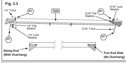
**D:** Attach 1 (H7) 1/4 x 5-1/2" Hex Bolt (with lock washer, flat washer and t-nut) to the ends of each (1826) Front Beam and (1825) Back Beam. The bolts do not attach to anything, but **MUST** be installed to the beams to prevent splitting and checking of wood. (fig. 3.2 and 3.3)
