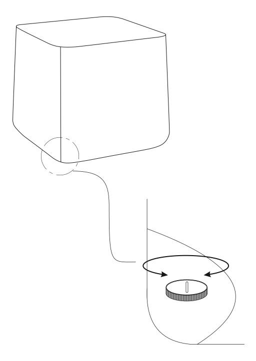
Note: Levelers on bottom of base can be adjusted if floor is uneven.
