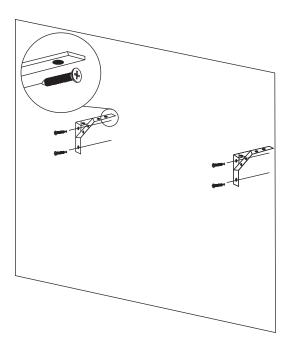
**2b.** • Place the countertop onto the mounting brackets. Apply silicone sealant to the mounting surface and press firmly.
