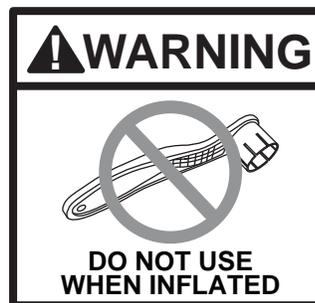
\*\*The Valve Wrench is to be used ONLY for tightening or changing the valve when the SUP is DEFLATED. It should NEVER be used when the SUP is inflated.
