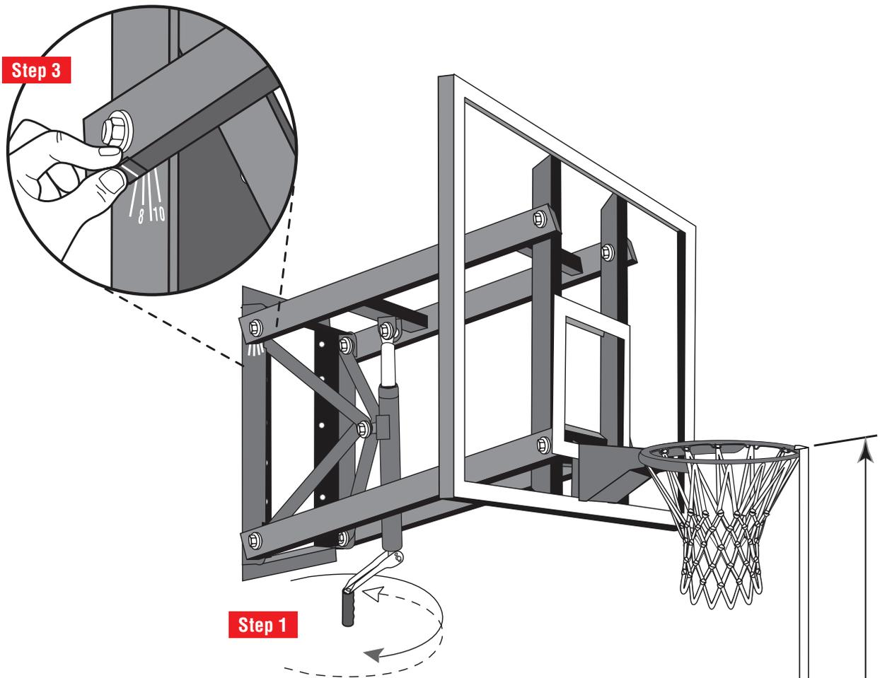
**Step 1:** Position top of rim 10' above playing surface by turning crank handle.
