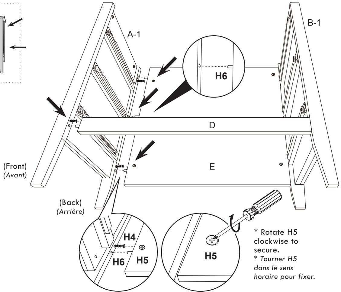
\* Rotate H5 clockwise to secure.
