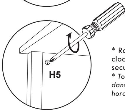
\* Rotate H5 clockwise to secure.
