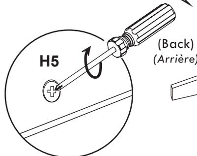
\* Rotate H5 clockwise to secure.
