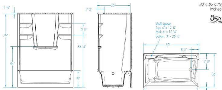
FEATURES Dimensional Tolerance ± 3/8". Dimensions needed for site preparation should be measured from the unit. Manufacturer assumes no responsibility for preparatory work.
