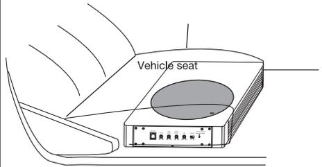
Make sure there is sufficient air circulation around the intended mounting location. Position the subwoofer enclosure where you wish to install it. Make some small marks to identify the position and remove the unit.
