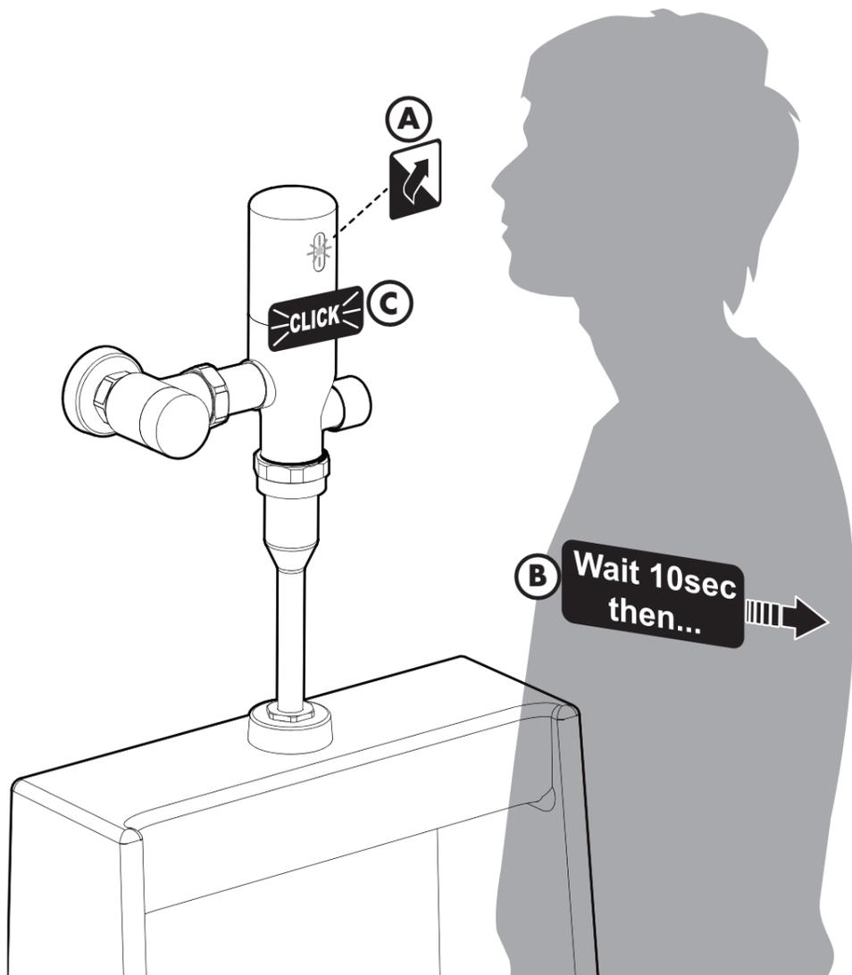
The factory set range is 25-1/2". Sensors in the wash closet models are pointed 15 degrees up, while urinal sensors are pointed 15 degrees down.
