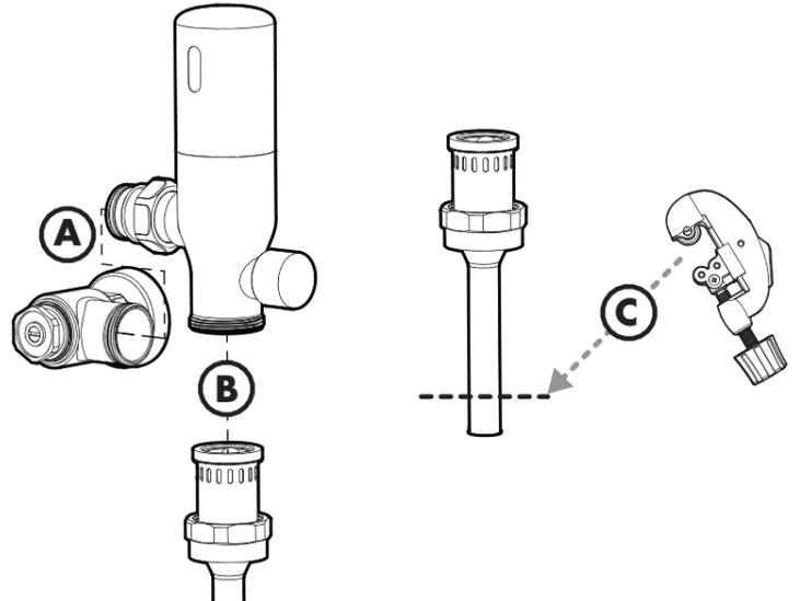
**NOTE:** Dry connections only! Do **NOT** use any thread sealant!
