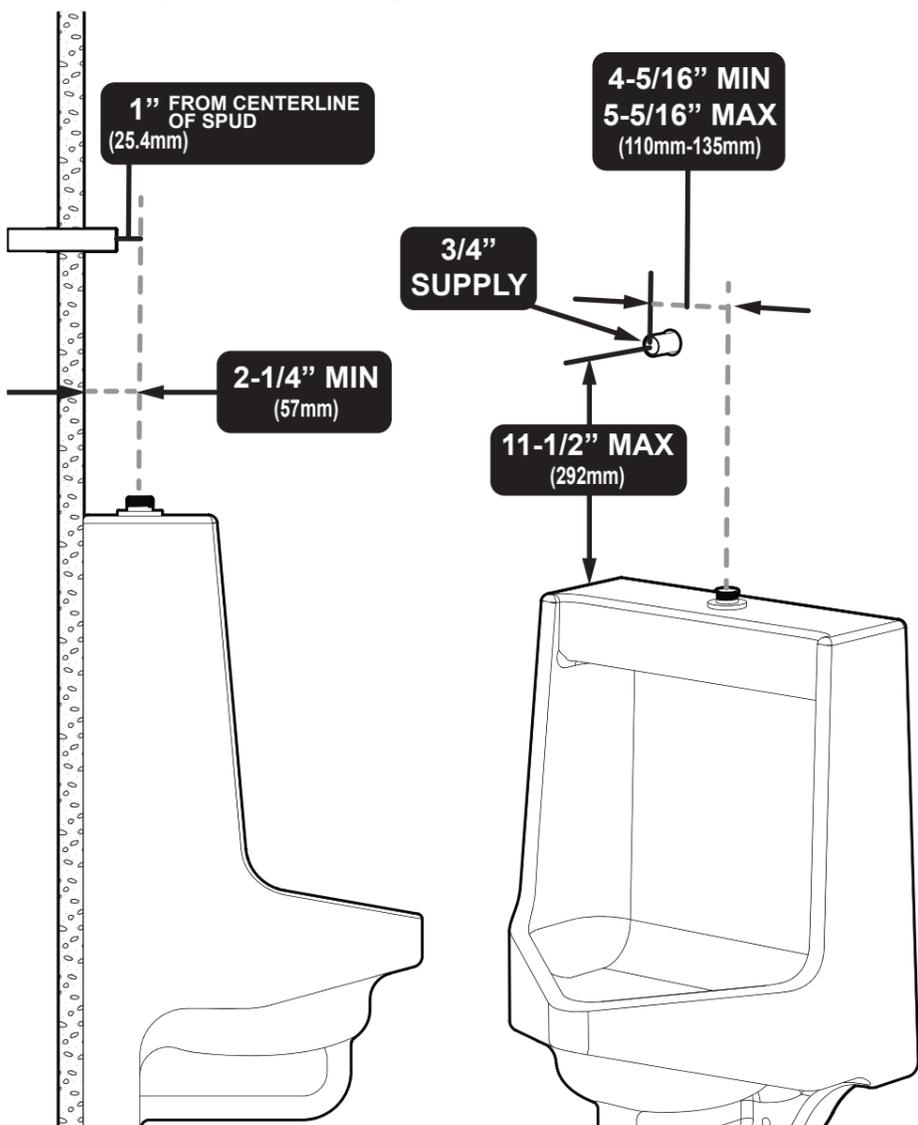
**NOTE:** If you are cutting the vacuum breaker tube to size, consult local plumbing codes to ensure that the critical line is properly located above the fixture. Typically, the critical line is 6" above the fixture.
