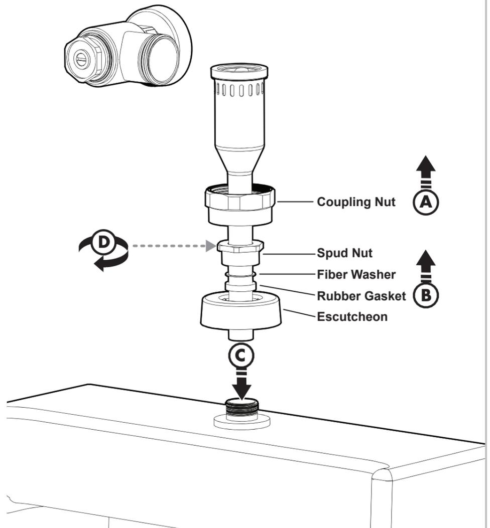
**NOTE: Dry connections only! Do NOT use any thread sealant!**
