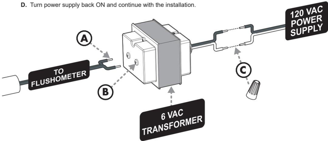
**NOTE:** Each flushometer requires 6 VAC of power and a between 0.35A and 0.5A of current to operate properly. 18-gauge wire is recommended to connect units. The number of Flushometers that can be wired in parallel depends on the capabilities of the sourced transformer. Example wiring diagram is below. Consult local electrical codes before installing.
