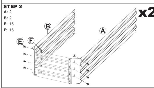
Ensuring the rolled edges are facing the inside of the garden bed, align one Long Panel (A) with the corner, as shown, and secure using four bolts and wing nuts.
