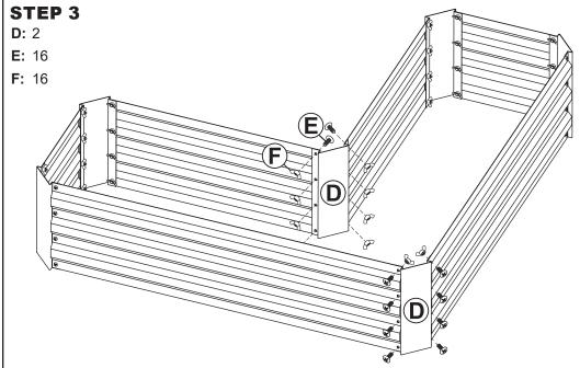
Loosely connect the long panels using one Corner (D), eight bolts and wing nuts.
