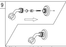
9. Attach screw onto hook ring as shown.
