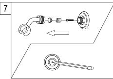
7. Remove sprayer hook ring from sprayer set and aim to required position on wall.
