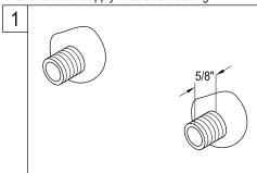
1. Plumb a 1/2"-14 NPT nipple protruding from the finished wall 5/8".
