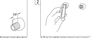
2. Turn on old faucet to remove any excess water in the supply lines. Apply Teflon tape onto both threads of supply elbows.
