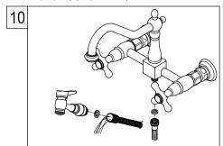
10. Remove spray head by unscrewing the sprayer in a counter clockwise direction, turn on both hot and cold valves and let water run for at least one minute, this will clear any debris left in the line.
