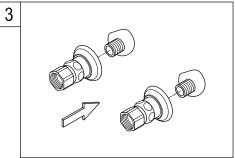
3. Remove elbow from faucet body and install to water outlet on wall.
