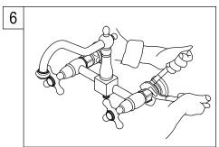
6. Install faucet body to supply elbows and tighten the elbow with an adjustable wrench.
