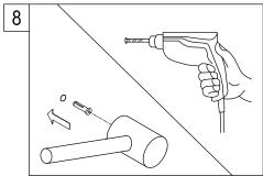
8. Insert anchor nut after hole drilling. (The size of the hole, anchor and screw must be properly proportional)
