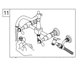
11. Remove aerator and turn on both hot and cold valves, let water run for at least one minute, this will clear any debris left in the line, reinstall aerator.
