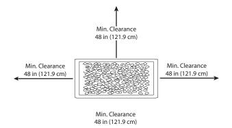
Combustible materials should not be within 72 inches of the top of the unit, or within 48 inches around the entire unit.
