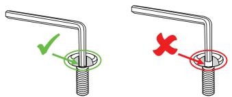
**TIP:** Always fully insert the hex key inside the designated notch of the bolt.
