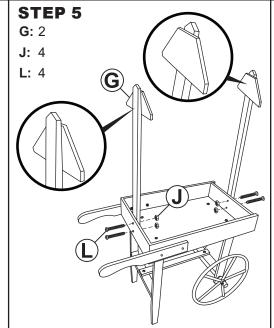
On the handle side, install one Support Post (G) on the inside of the planter box using two Bolts (L) and two Nuts (J).
