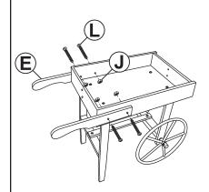
Firmly secure two Handles (E) to the planter box using two Bolts (L) and two Nuts (J).
