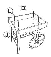
Align Planter Box (D) with the leg panels and loosely secure using four Bolts (L) and four Nuts (J).
