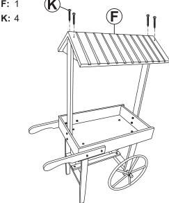
Place Roof (F) on the support posts and secure using four Screws (K).
