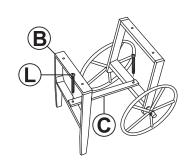
Fasten Support Bar (C) to the back leg panel using one Bolt (L).
