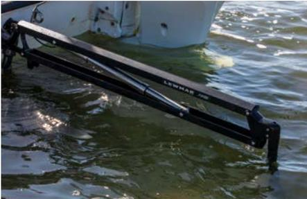
Lewmar shallow water anchors do not require hydraulic pumps or hoses, making them low-maintenance and easily installed
