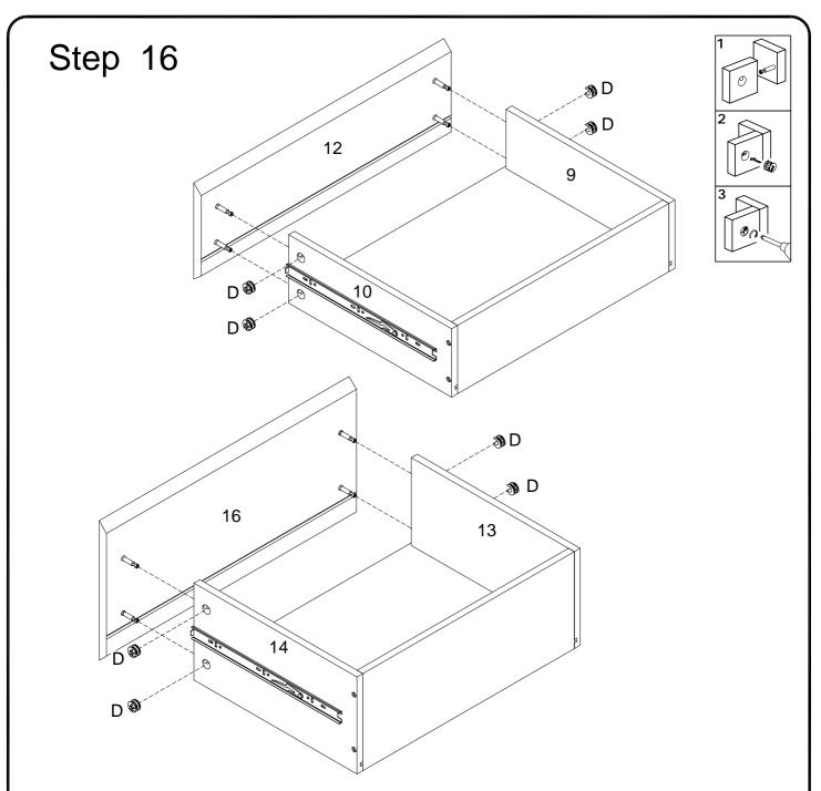
Using cam lock(D) secure part (12) into parts (9,10),part (16) into parts (13,14) with Philips head screwdriver as per diagram.
