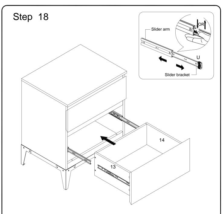
Insert the assembled drawers into the unit frame, extend the Ball Bearing Slide Tracks (U) on the pedestal Side Panel all the way forward .Then align the Slide Runners on the assembled drawers with the Slide Tracks and push the drawer carefully inside until it stops.
