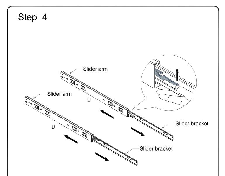
Pick up the slider arm (U) and separate the slide Runner for the following Steps. Extend the Slide .Runner all the way forward, press the plastic release lever of the alider arm up and pull the Slide Runner Complete out .
