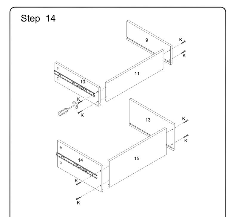
Using screw (K) attach parts (9,10) to part (11),parts (13,14) to part (15) with Philips head crewdriver as per diagram.
