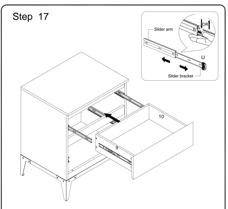
Insert the assembled drawers into the unit frame, extend the Ball Bearing Slide Tracks (U) on the pedestal Side Panel all the way forward .Then align the Slide Runners on the assembled drawers with the Slide Tracks and push the drawer carefully inside until it stops.
