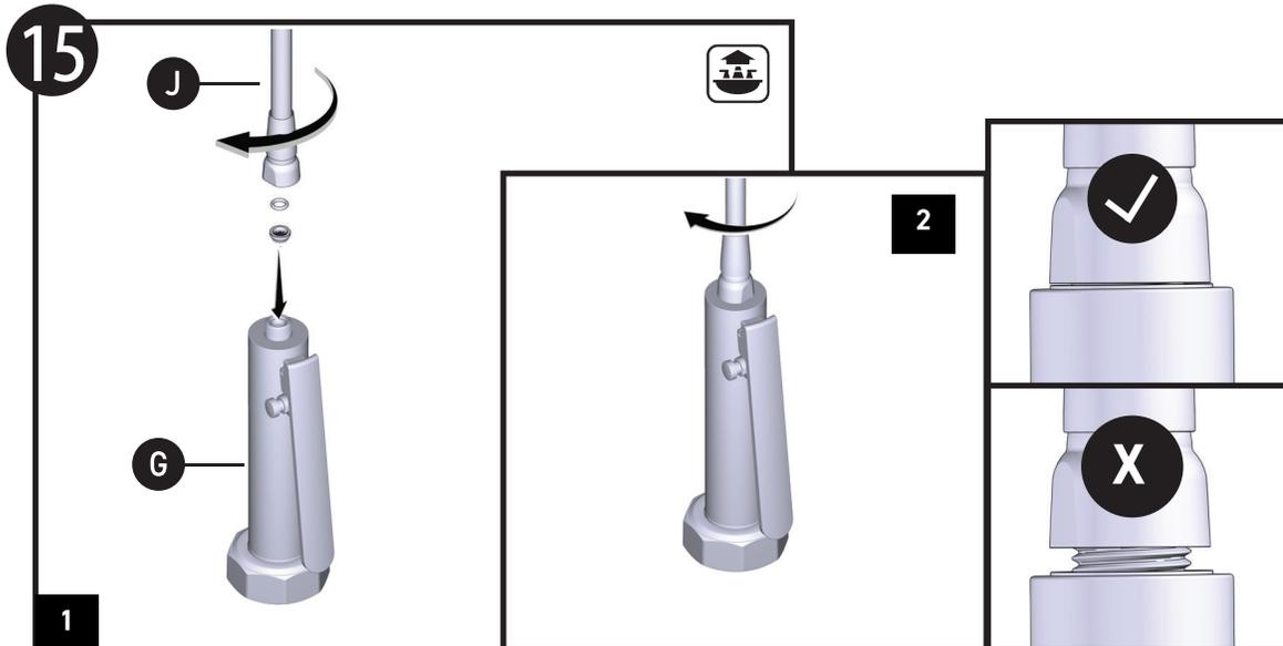
1. Reinstall screen and o-ring as shown. Thread Pulldown Hose (J) onto Spray Wand (G) and tighten. Tighten Pulldown Hose (J), flush with Spray Wand (G). Do not overtighten.
