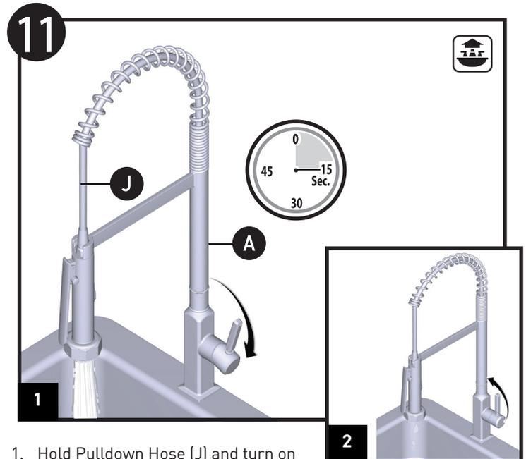
1. Hold Pulldown Hose (J) and turn on Faucet (A), allow water to run for 15 seconds.
