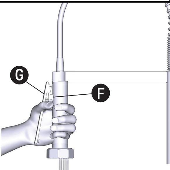
Wand will now be back in Low Flow mode. Note: Wand will also revert to Low Flow mode when water is shut off.
