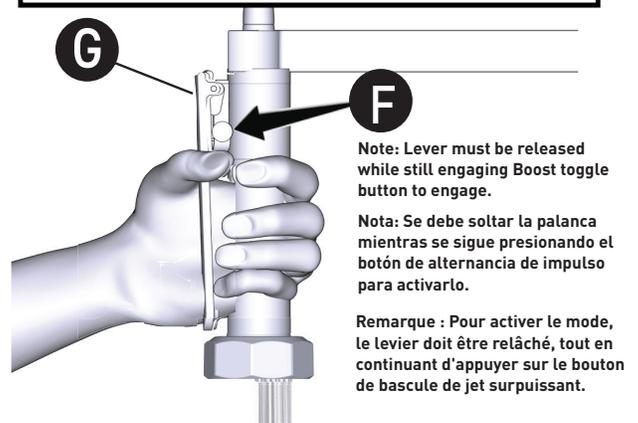
Note: Lever must be released while still engaging Boost toggle button to engage.
