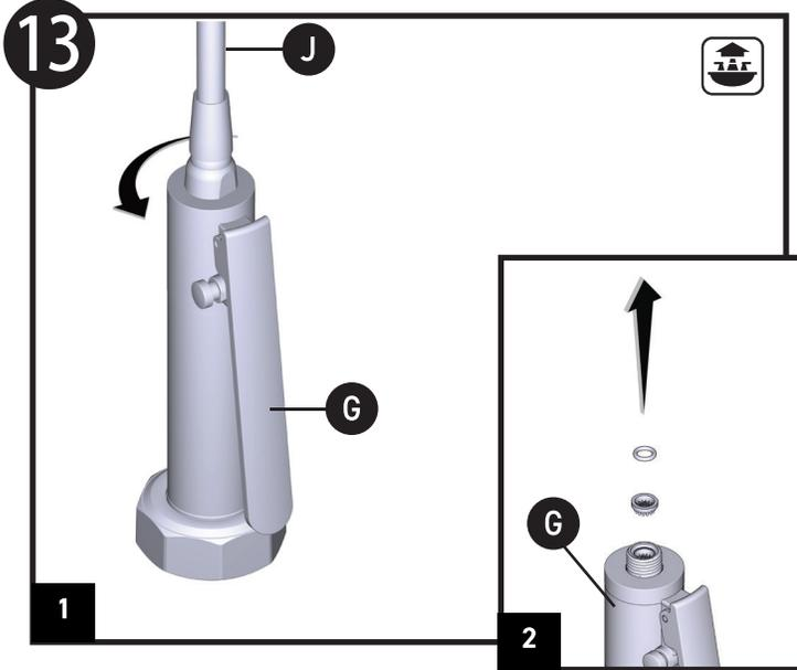
1. Unscrew Pulldown Hose (J) from Spray Wand (G) and remove screen and o-ring.
