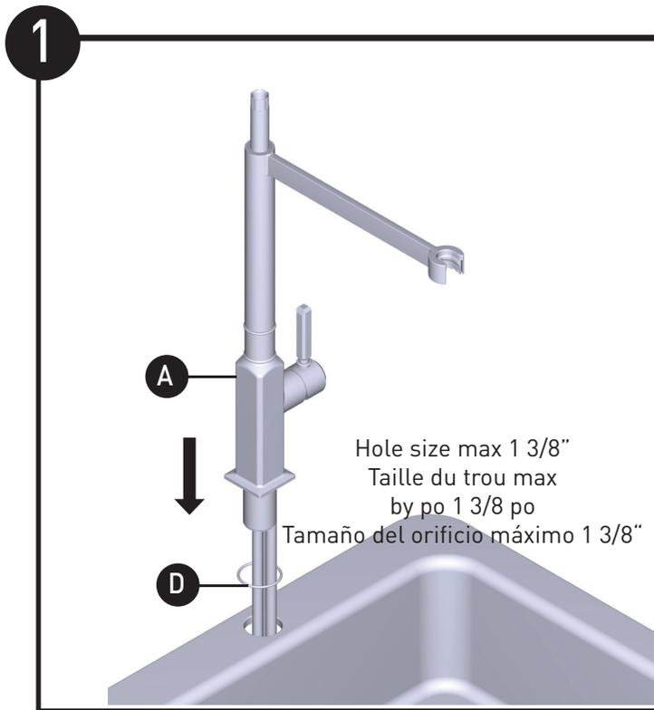
1. Place O-ring (D) onto base of Faucet Body (A) aligning ribs on faucet (if present) to slots on O-ring (D). Place into sink hole. NOTE: Install with handle on right side only.
