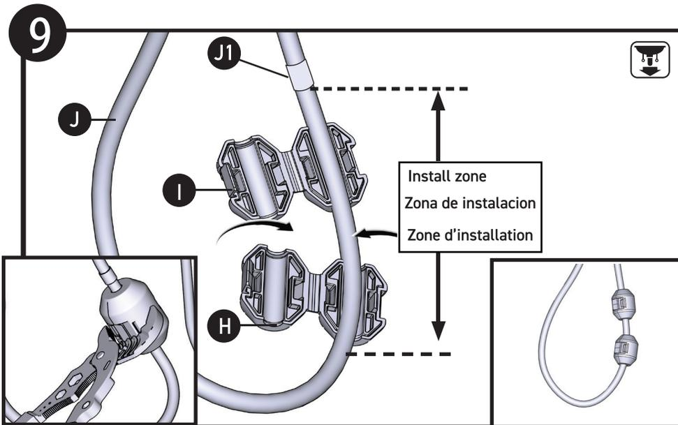
**IMPORTANT** - Locate Hose Weight Locator Mark (J1) on Pulldown Hose.(J) Install Hose Weight (H&I) just above of loop curvature in hose on same side of hose as locator mark.
