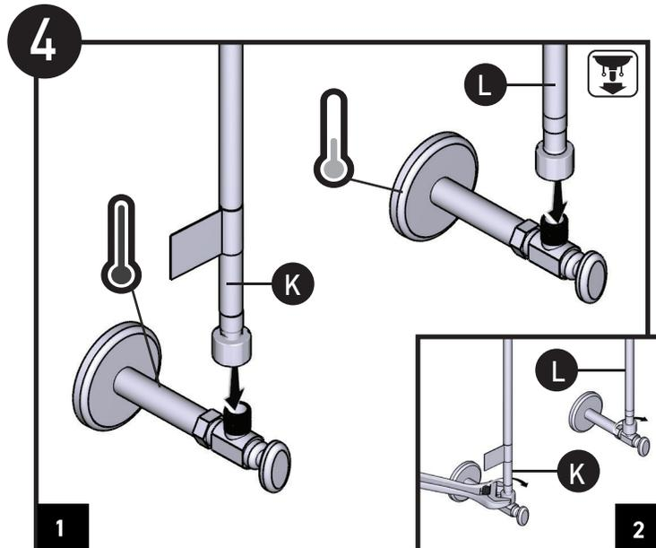
1. Attach Flexible lines (K and L) to shutoff valves.
