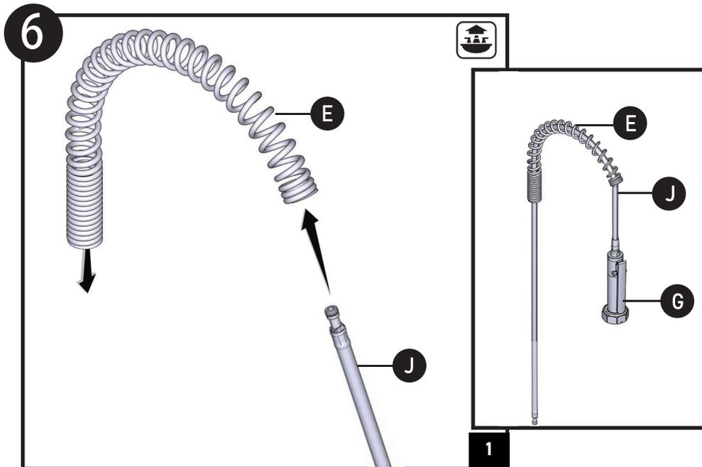
1. Insert small end of Pulldown Hose (J) into spout and feed through Coil Spring (E).
