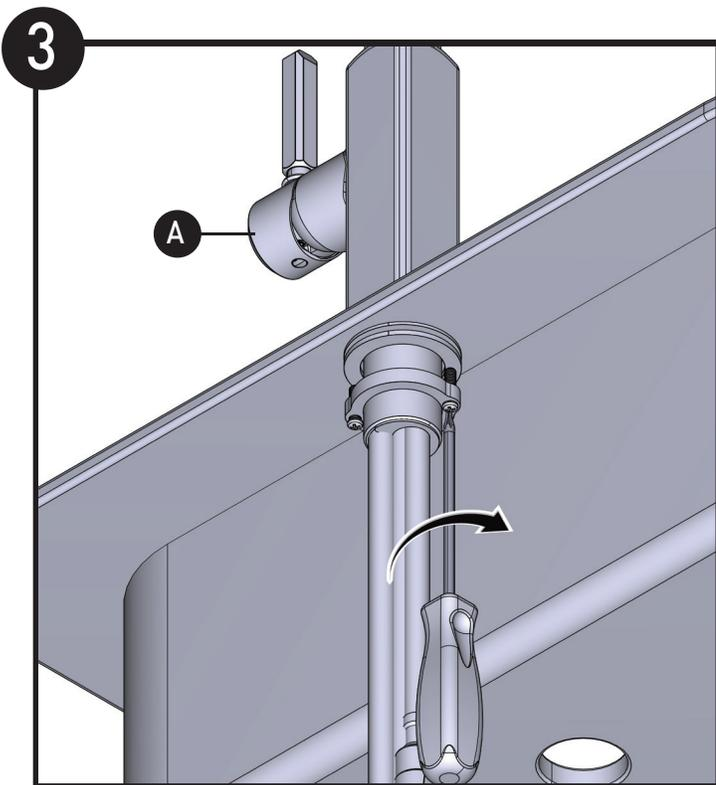
Tighten screws of Below Deck Mounting Hardware (C) with a screwdriver.
