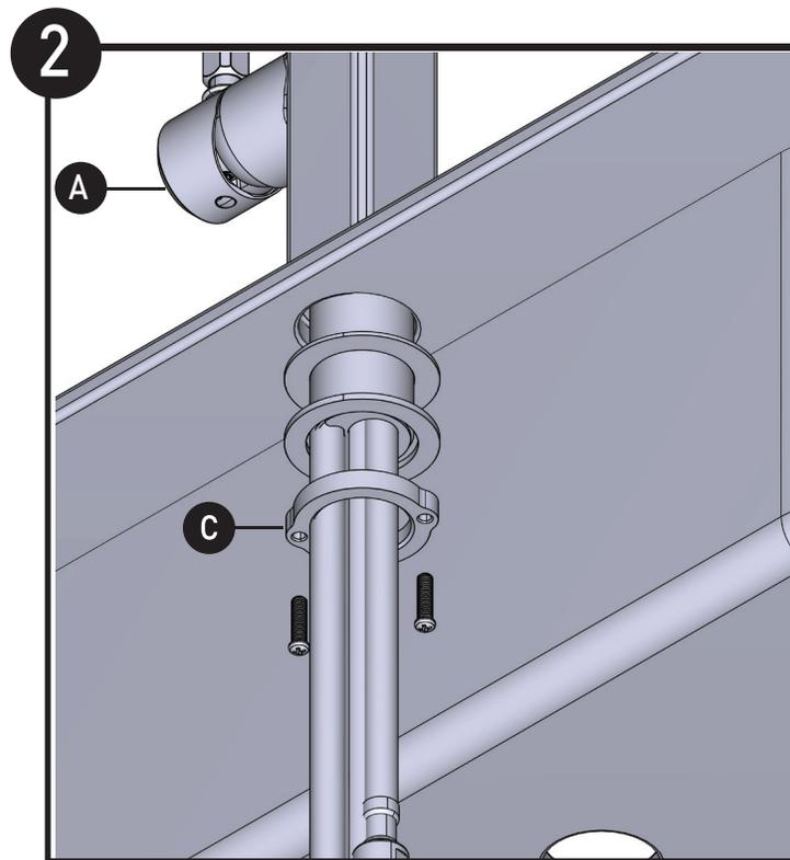
Install the Below Deck Mounting (C) onto threads of the Faucet Body (A).
