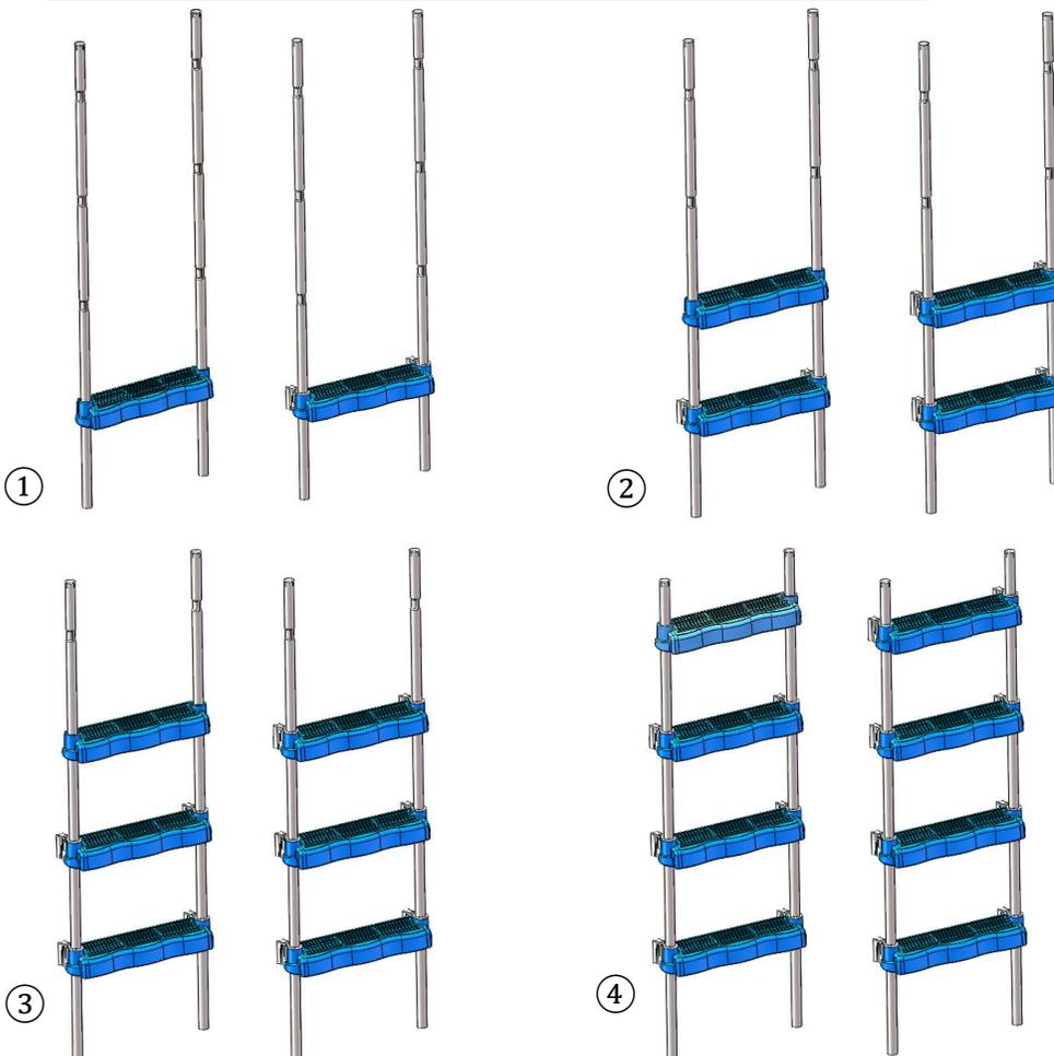
Follow **ASSEMBLY DETAIL A** to install the Steps and then Follow **ASSEMBLY DETAIL B** to install two bushings on as shown in sub-steps ① through ④, above. For easier installation, remove the White Plugs first and when the bushings are installed, re-install the white plug.
