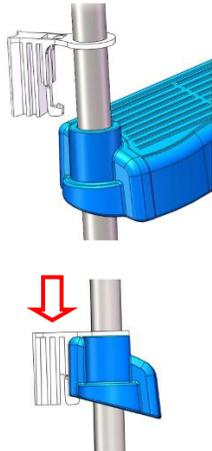
**ASSEMBLY DETAIL B** – Detail Diagrams of Bushing installation
