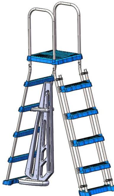
① Insert the removable Safety Steps into the holes in the Bottom Outside Step. Tilt the Removable Safety Steps up, aligned with the Outside Rails.
