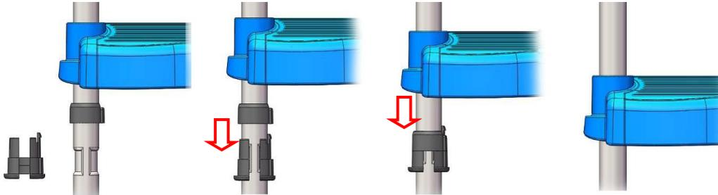
**ASSEMBLY DETAIL A** – Detail Diagrams of Step/Platform installation
