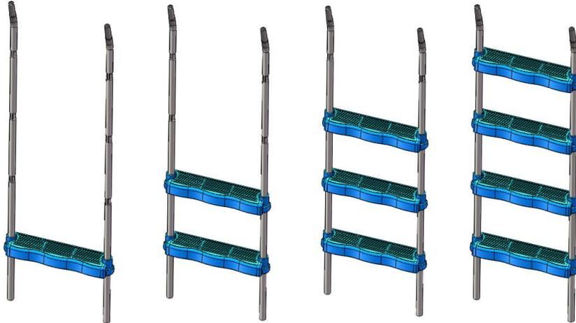
Follow **ASSEMBLY DETAIL A** to install the first step through the fourth step of inner ladder.
