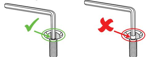
If the hex key is not fully inside the notch, the hex key could slip out, causing damage to the bolt head. Repeated hex key slipping will cause the notch to become rounded, making it difficult or impossible to tighten the bolt with the hex key.
