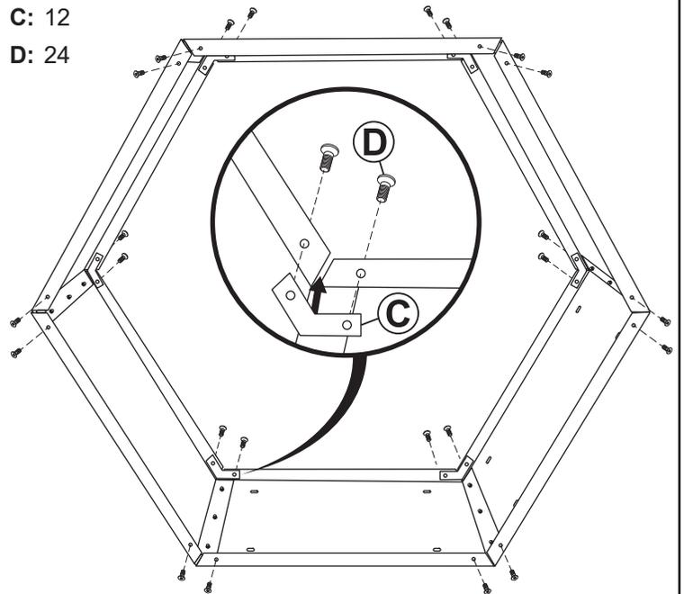
Loosely secure one Bracket (C) onto each inside corner using two M6x10mm Bolts (D).
