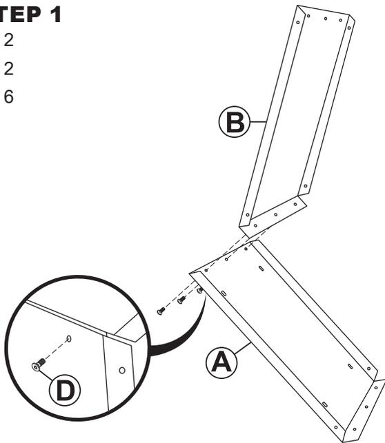
Align the lip of one Solid Panel (B) with the inside of one Expansion Panel (A) and loosely secure using three M6x10mm Bolts (D).
