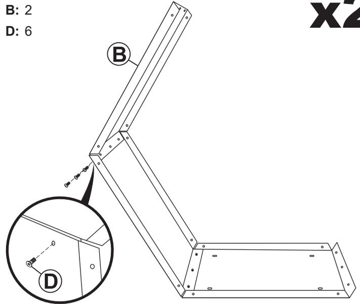
Align the lip of one Solid Panel (B) with the inside of the solid panel from the previous step and loosely secure using three M6x10mm Bolts (D).
