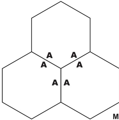
Position each unit with Expansion Panels (A) aligned as shown.
