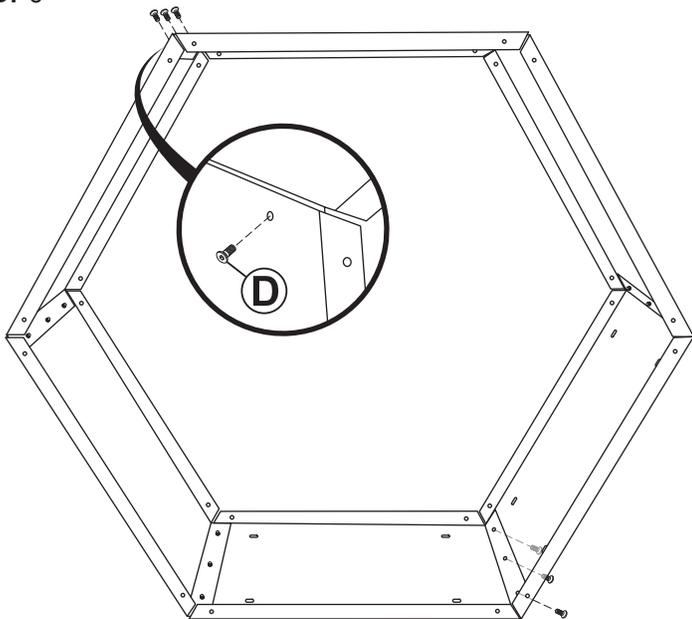
Align the expansion panels and the solid panels. Then, loosely secure using six M6x10mm Bolts (D).
