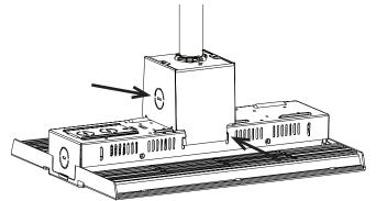
3 Route wiring through the pendant box, end plate knockout, and fixture wire cover. Make sure to adequately protect the wiring. Make wiring connections per the wiring diagram.
