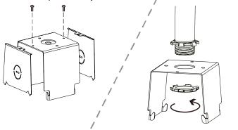
2 Insert the tabs of the pendant box into the corresponding slots of the fixture junction box. Remove the knockout of the plate.
