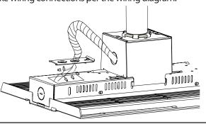
4 Secure end plates onto pendant box with provided hardware.
