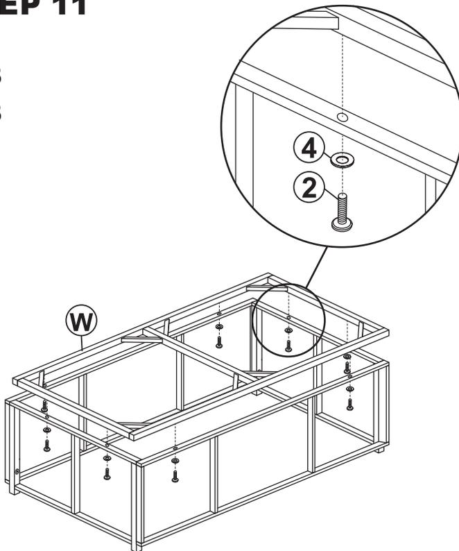
Do not fully tighten hardware until all components in this step have been connected.
