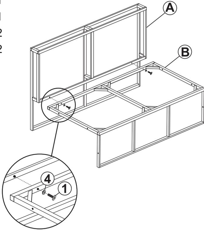
Do not fully tighten hardware until after Step 3 is complete.
