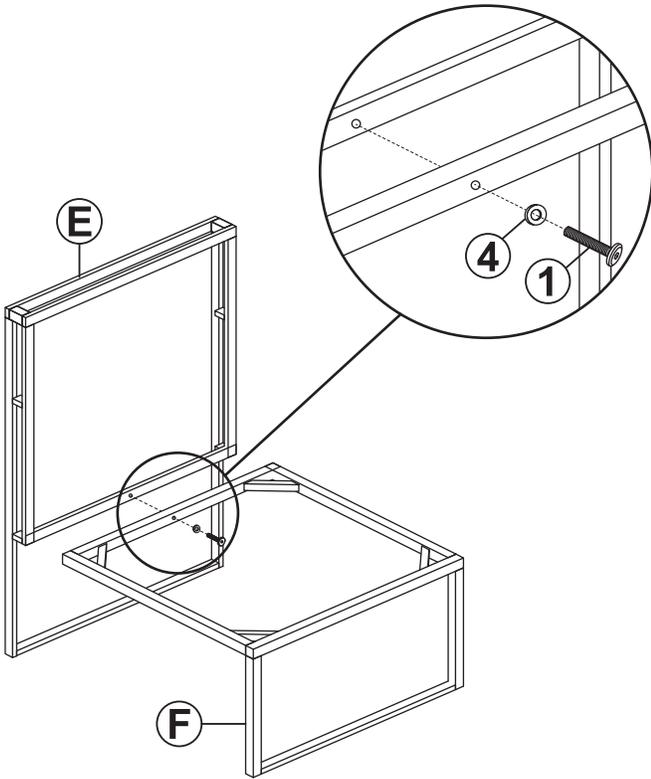
Do not fully tighten hardware until after Step 7 is complete.
