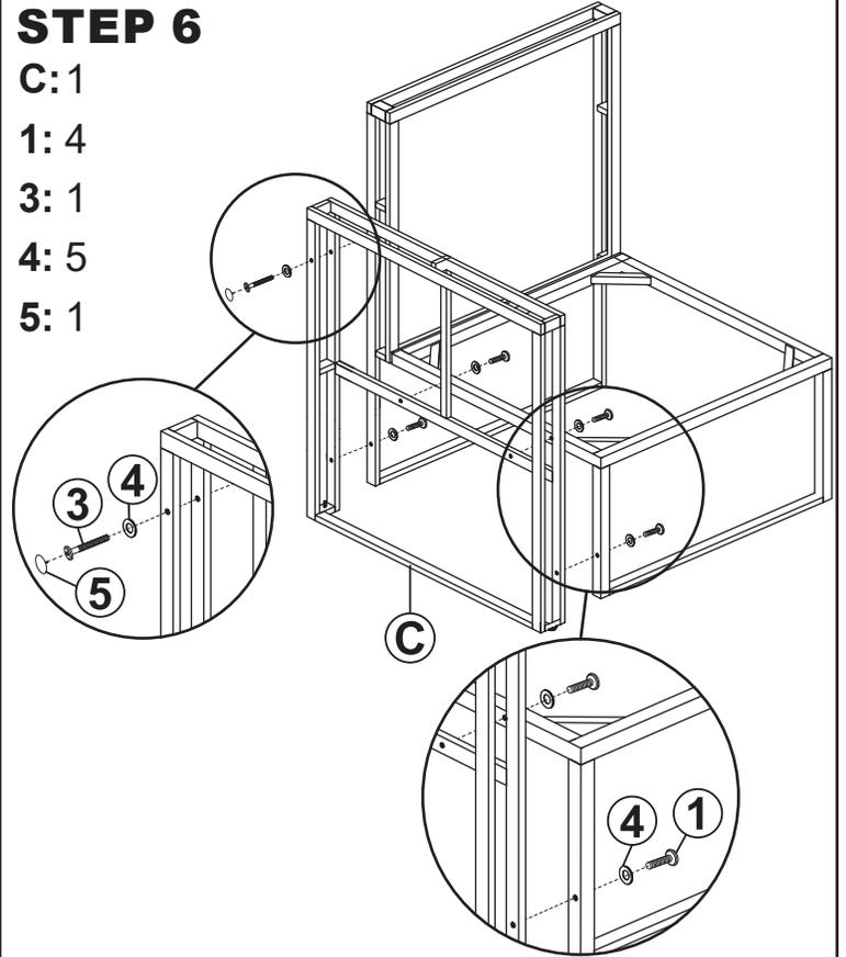
Do not fully tighten hardware until after Step 7 is complete.
