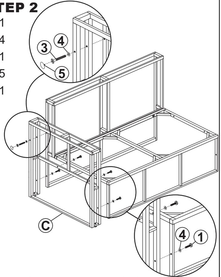
Do not fully tighten hardware until after Step 3 is complete.
