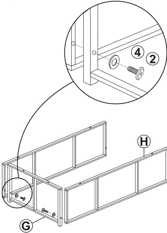
Do not fully tighten hardware until after Step 11 is complete.
