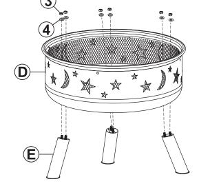
Install Legs (E) to Fire Bowl (D) using Washers (4) and Nuts (3).
