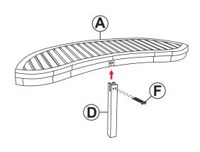
Secure Leg (D) to the front of Seat (A) using two 4cm Bolts (F).
