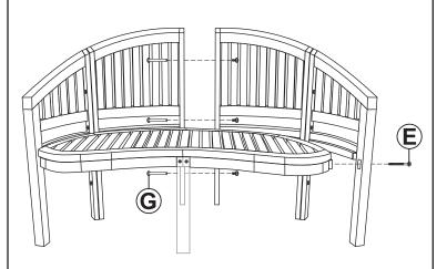
Loosely secure the left backrests to the seat using one 5cm Bolt (E). Then firmly secure the inside backrests using three 5cm Chicago Bolt Sets (G).
