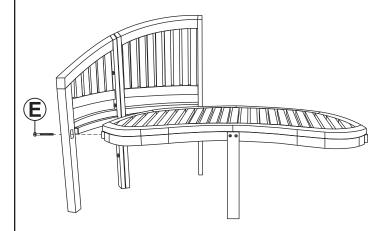
Loosely secure the seat to the right backrests using one 5cm Bolt (E).
