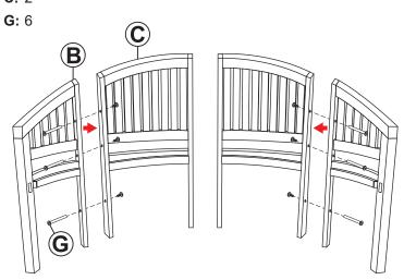
Loosely secure the right Outside Backrest (B) to the right Inside Backrest (C) using three 5cm Chicago Bolt Sets (G).
