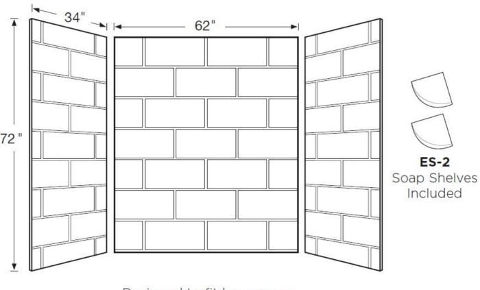
Designed to fit base areas 34" deep or smaller x 62" wide x x 72 ½" high or smaller (864 mm x 1575 mm x 1829 mm)
