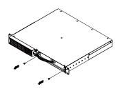
3. Remove two retaining screws, pull out the old battery pack and replace new one. Reassemble the retaining screws, covers, black and red cable, and front panel in the reverse sequence of the above steps. Recharge the unit for at least 8 hours with the unit turned on or at least 24 hours with the unit turned off to ensure maximum UPS battery runtime.
