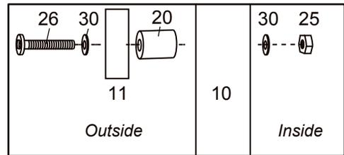
Hinge / Leg Support Assembly (both sides)
