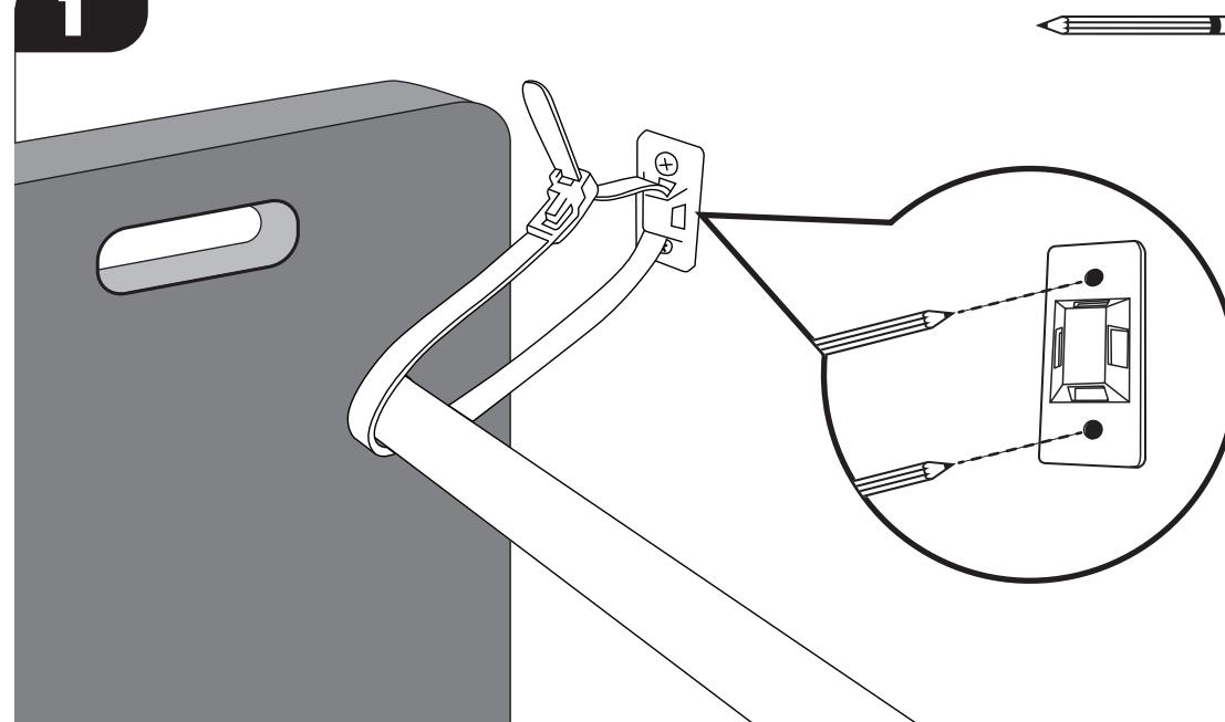
**DRY WALL INSTALLATION:** Place the assembled organizer against the wall. Use the Mounting Bracket as a guide to mark drill-holes on the wall, at the same height as the top support bar. Do this for left and right side of the organizer. Consult with a professional if you require an installation other than dry wall.
