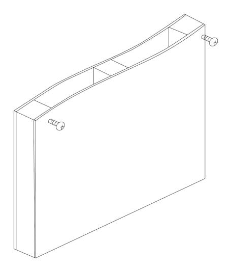
Drill at marked locations using 3/32-in. diameter drill bit (not included). Insert appropriate screws or wall anchors (not included) into holes. NOTE: Be sure the hardware is rated to handle appropriate weight of the mirror.
