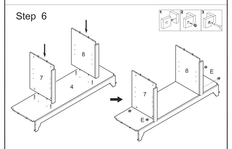
Attach panels (7,8) to bottom panel (4) using cam bolts and dowels as guides. Insert cam locks (E) into panels (7,8) and tighten with a screwdriver.
