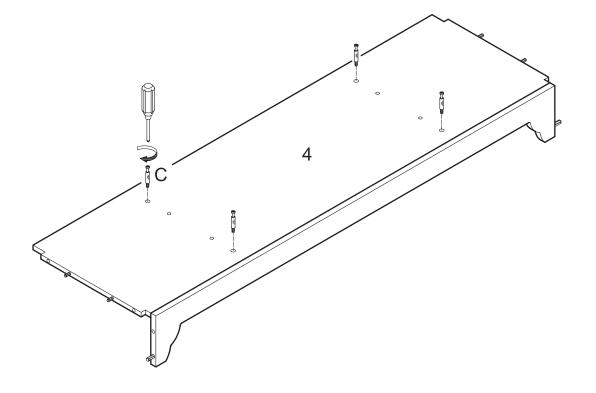
Screw cam bolts (C) into bottom panel (4).
