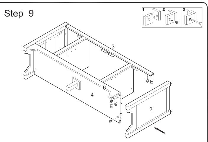
Attach side panel (2) to the opposite side of the assembly from Step 7 using cam bolts and dowels as guides. Insert cam locks (E) into bottom panel (4) and slats (3,6). Tighten cam locks (E) with a screwdriver.
