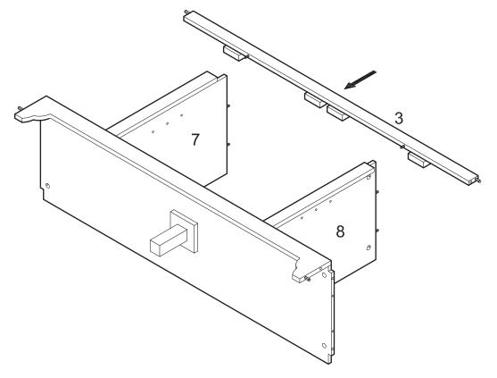
Attach slat (3) to panels (7,8) using dowels as guides.
