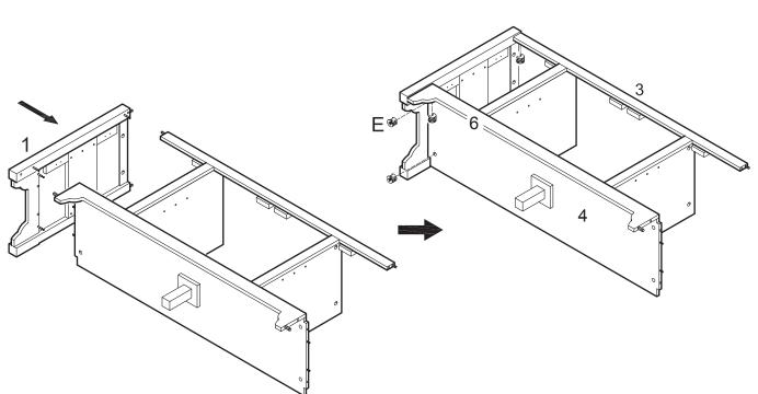
Attach side panel (1) to the assembly from the previous step using cam bolts and dowels as guides. Insert cam locks (E) into bottom panel (4) and slats (3,6). Tighten cam locks (E) with a screwdriver.
