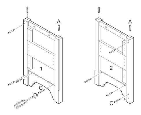
Insert large dowels (A) into side panels (1,2). Screw cam bolts (C) into side panels (1,2).
