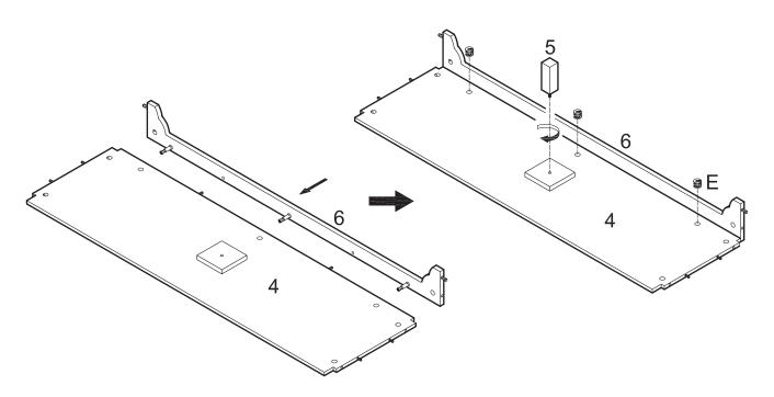
Attach slat (6) to bottom panel (4) using cam bolts and dowels as guides. Insert cam locks (E) into bottom panel (4) and tighten with a screwdriver. Screw leg (5) into bottom panel (4).
