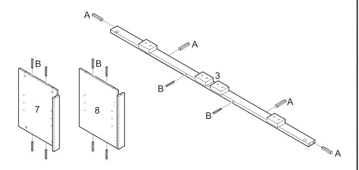
Insert small dowels (B) into panels (7,8) and slat (3). Insert large dowels (A) into slat (3).
