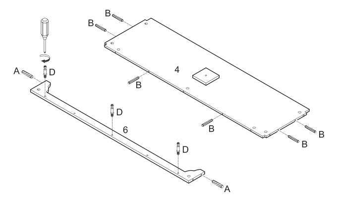
Insert large dowels (A) into slat (6). Insert small dowels (B) into bottom panel (4). Screw cam bolt (D) into slat (6).
