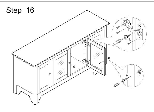
Attach doors (14,15) to the stand assembly using medium screws (M) at the hinges. Attach handles (G) to doors (14,15) using bolts (H).
