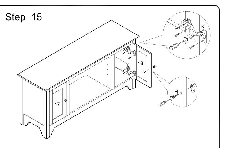
Attach doors (16,17) to the stand assembly using medium screws (M) at the hinges. Attach handles (G) to doors (16,17) using bolts (H).
