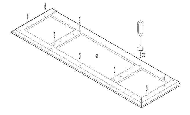
Screw cam bolts (C) into top panel (9).
