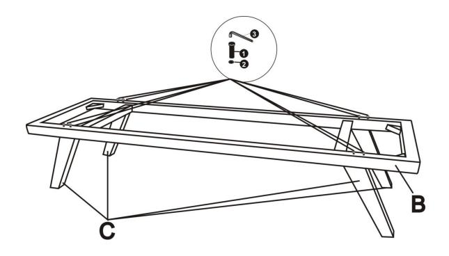
Attach Legs (C) to Apron (B) with Allen Key Screws (1) and Washers (2). Use Allen Key (3) to fully tighten all Screws.
