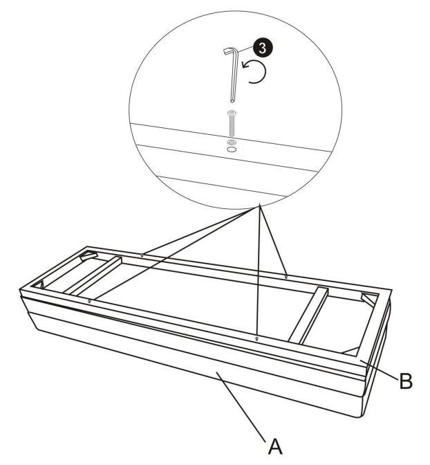
Remove pre-assembled Allen Key Screws (1) and Washers (2) from Apron (B).
