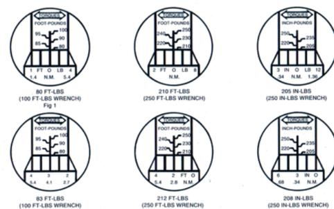
\* Various models and capacities of wrenches are illustrated. Though they might be different from your particular wrench, the principle of obtaining scale reading is the same.
