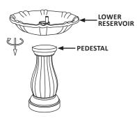
**2.** Feed the pump cable through the plastic tube in the reservoir, and through the channel on bottom of the pedestal.
