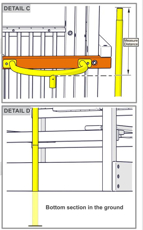
**5.** Insert the top part of the Pole into the mounting tube and fasten with two 1/4"lock washers **PG-HW-W013** and two button head screws **PG-HW-B023** as shown in **Detail E**.
