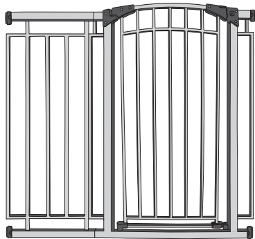
3 38.25 - 43.50 in. (97.1 - 110.5 cm) with Long Frame Extension
