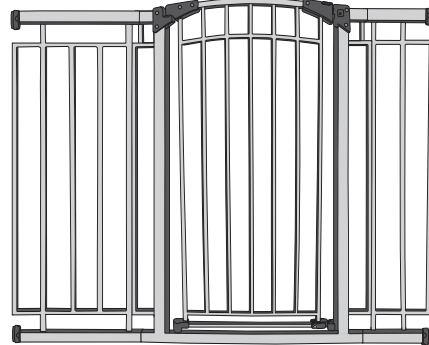
4 43.50 - 48 in. (110.5 - 121.9 cm) with Short and Long Frame Extensions
