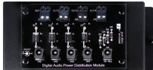
Digital Audio Power Distribution Module PW1020
