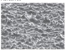
Variable and sized randomly arranged minerals leave inconsistent finish with deep scratches that are hard to buff. 3M™ Trizact™
