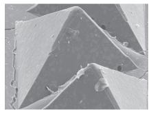
Uniform size distributed abrasive structures provide uniform patterns and consistent sand scratches for leveling imperfections and defects.
