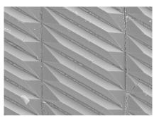
For an even finer sand scratch, elongated distributed abrasive structures are used to provide uniform patterns and consistent sand scratches. This allows for faster buffing and better finishes.
