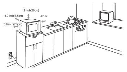
A minimum clearance of 3.0 inches (7.5cm) is required between the oven and any adjacent walls. One side must be open.
