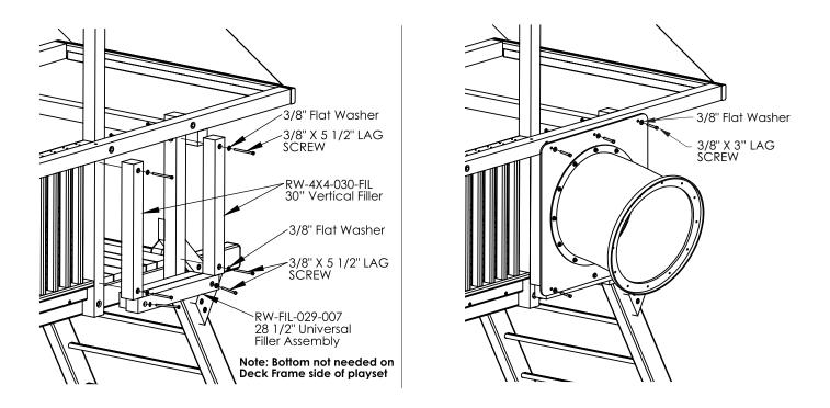
**4.** Assemble remaining slide sections as shown on the assembly page for your application.
