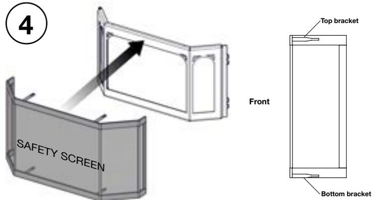
Ensure safety barrier is installed correctly. Note the orientation illustrated.
