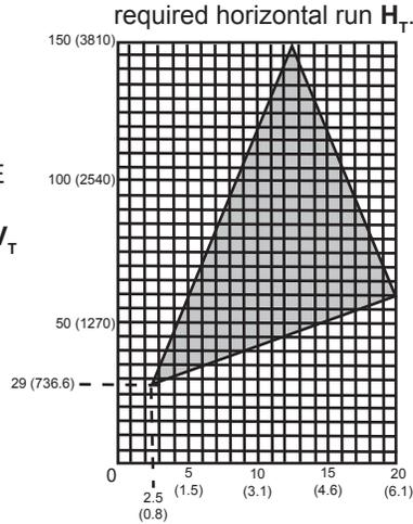
HORIZONTAL VENT RUN PLUS OFFSET IN FEET (METERS)  $H_T$
