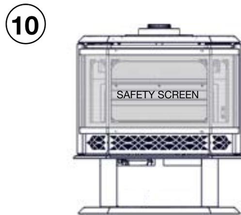
When opening the fire viewing door, a simple procedure must be followed in order to not damage the door. First open the valve control door. Next open both side doors fully. Pull the latch handles towards you and release each catch. The door may now be safely opened. To close the door, repeat in reverse order.
