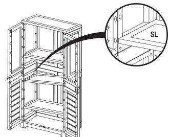
Install Shelves (SL) into the unit at a slight angle and align the shelf with one side of the unit. Then, gently press on the opposite side down until the shelf locks into place.
