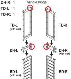
Assemble the doors as shown: Top door, handle, bottom door.
