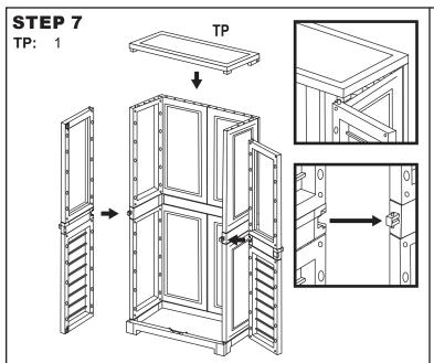
Affix the backside of Top Panel (TP) to the back and side panels; do not affix the front of the top panel.
