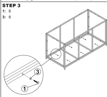
Do not fully tighten hardware until after step 5 is complete.
