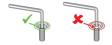
If the hex key is not fully inside the notch, the hex key could slip out, causing damage to the bolt head. Repeated hex key slipping will cause the notch to become rounded, making it difficult or impossible to tighten the bolt with the hex key.
