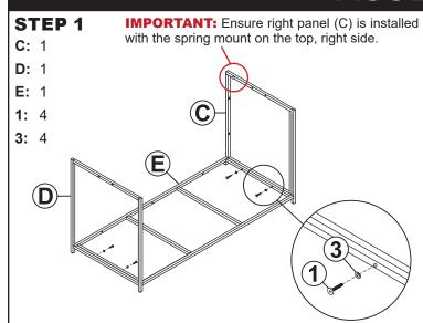
Do not fully tighten hardware until after step 5 is complete.
