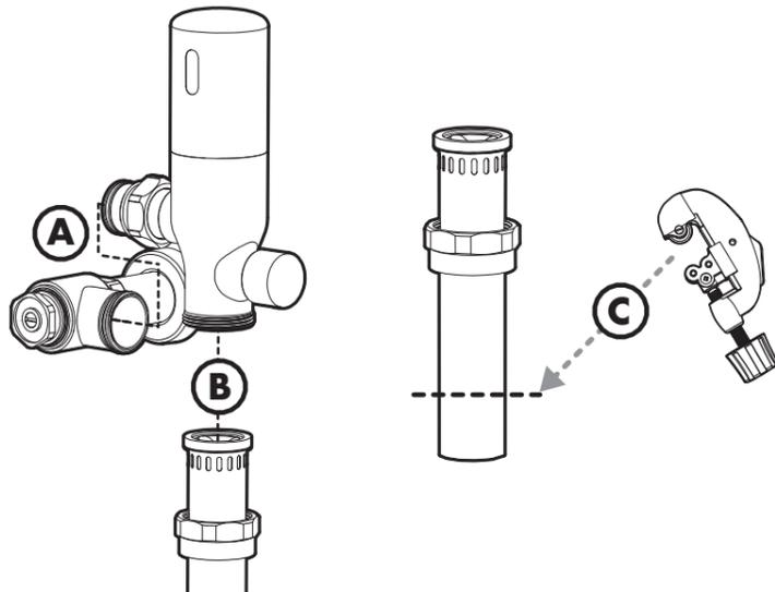
**NOTE:** Dry connections only! Do **NOT** use any thread sealant!
