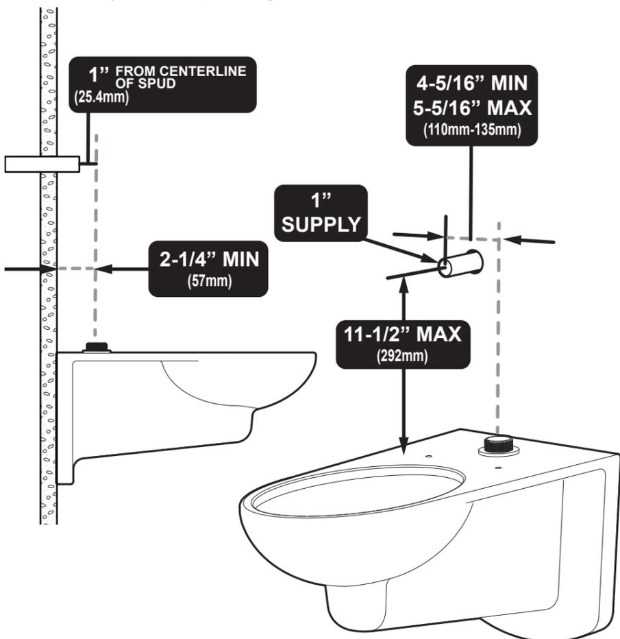
**NOTE:** If you are cutting the vacuum breaker tube to size, consult local plumbing codes to ensure that the critical line is properly located above the fixture. Typically, the critical line is 6" above the fixture.
