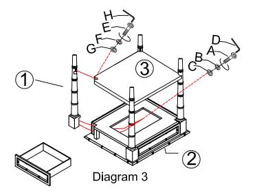
Step 3: Assemble the rest of the leg to the top and bottom shelf (Refer to Diagram 3).
