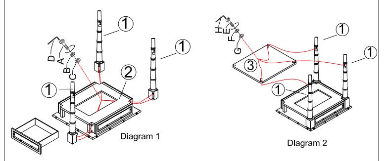
Step 1: Attach three of the legs (1) to top (2), well insert bolts (A), lock washers (B) and flat washers (C). Please do not fully tighten bolts. (See Diagram 1)
