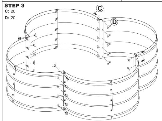
Align the four sets of panels and loosely fasten each section using the remaining Bolts (C) and Wing Nuts (D), as shown.
