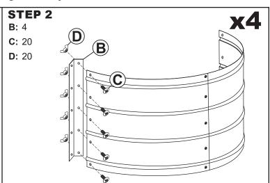
Align one Corner (B) with the left side of one of the assembled panel sets.
