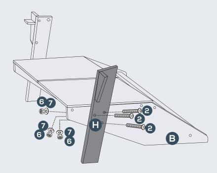
Attach Part E Left Chair Arm to Part H Left Chair Leg with 1 set of Hardware #1 Bolt, #7 Washer and #6 Nut.
